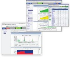
GE's iUPSGuard is a remote monitoring solution for UPS, providing status monitoring and alarm notification that supports all GE UPS product lines, anytime, anywhere. iUPSGuard provides current and detailed information about UPS operation, including its configuration, internal alarms, automatic reporting and operating conditions over the web.
