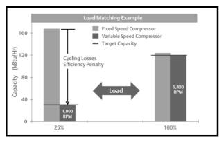
VFD Advantage 2 – Better temperature control compare to normal fix speed control.
