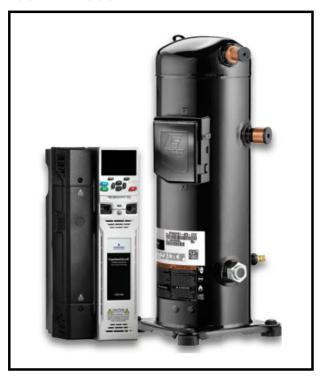
DB-Aire III offers the Variable Frequency Drive (VFD) compressor to satisfy the needs of high efficiency and low energy product. The capability to modulate the compressor speed will allow it to match the on-demand capacity while maintaining the optimum power usage. Significant energy saving can be expected during part load condition. The low start-up frequency is also contributing to the lower initial current peak that usually happen in conventional fix speed compressor.
