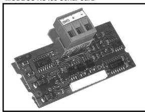
Optional Modbus RS485 add-on card allows Vision 2020i Controller to interface to Modbus Slave, RTU mode, RS485 network. The maximum rate is 19200 and it is set via software.
