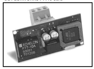
The optional Lonworks serial card allows Vision 2020i controller to interface to LonWorks® network FTT-10A 78 kbs (TP/FT-10).
